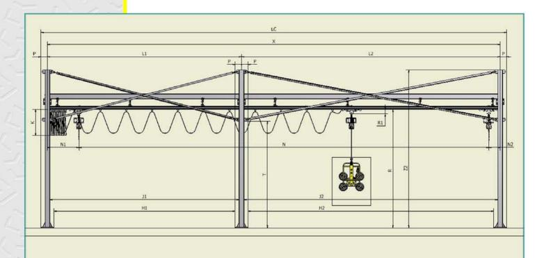
Overhead suspended rail with vacuum lifter
