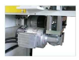
Z-axis controlled by PC automatic adjustment of screwing heads distance
