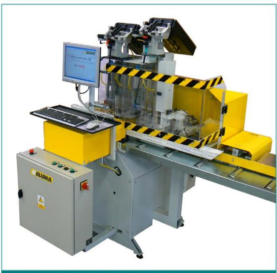
CYKLON D - Two-head reinforcement screwing unit
