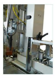
Pneumatic length stop for profile insertion adjustable in accordance with screwing instruction about position of the first screw
