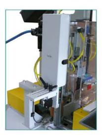
Pneumatic length stop for profile insertion adjustable in accordance with screwing instruction about position of the first screw
