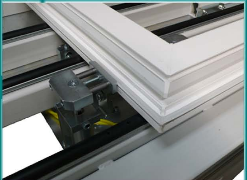
Reading assessment right and left, pneumatic lowering for the fitting length calculation
