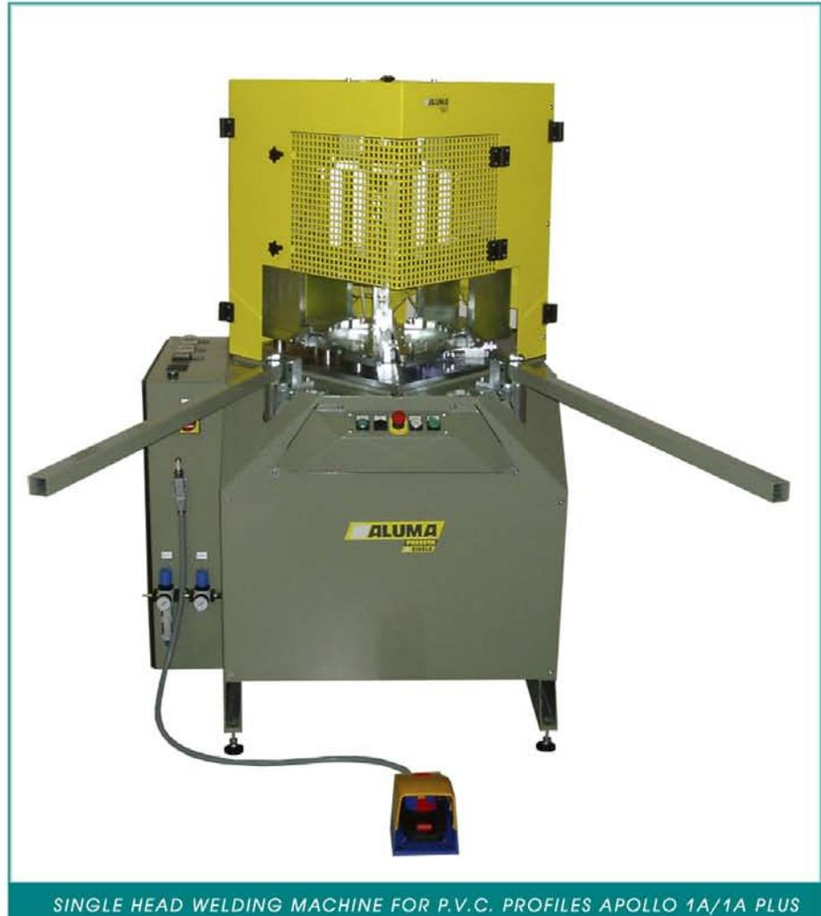
SINGLE HEAD WELDING MACHINE FOR P.V.C. PROFILES APOLLO 1A/1A PLUS
